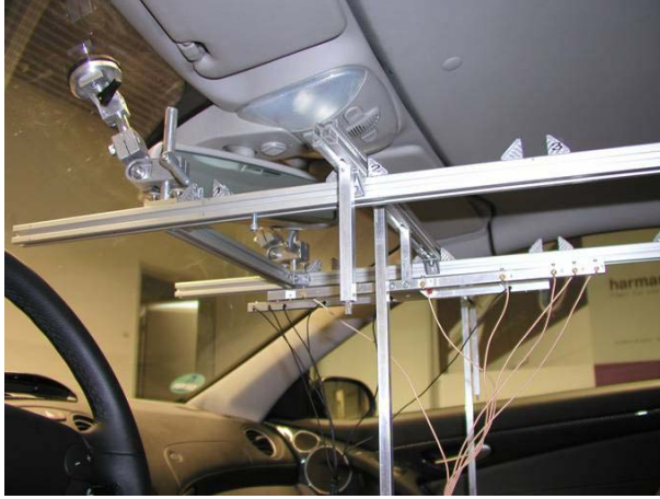
Figure 26. 12-microphones array and carrier embodiment.
